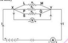
It is observed that the total current, I is equal to the sum of the separate currents through each branch of the combination.
